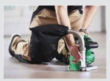
Step 1: Milling the groove with the GROOVER.
