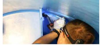
WELDING PEN R combined with angle adapters make welding possible even in very tight spaces.
