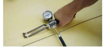
Testing the leak-tightness of lap seams with test channel.
