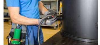
LABOR S, used in combination with MINOR as an external air supply.
