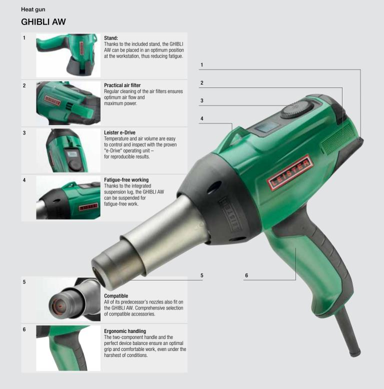
practical device suspension make working easier. The air filters can be readily removed and cleaned. And of course, all of the nozzles from its predecessor fit the new GHIBLI AW.
