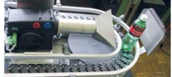
HOTWIND SYSTEM with wide slot nozzle integrated in a blow-off application.
