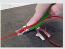
Step 4: Levelling the protruding welding rod with Quarter Moon Knife or Trimming knife.
