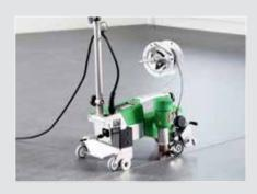
Step 2: Inserting the welding rod into the groove with the UNIFLOOR E hot-air welder.
