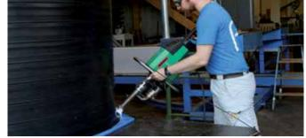
The WELDPLAST S6 is guided easily with the practical control wheel grip.
